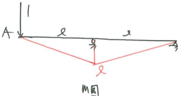
$$\Delta A = \left(\frac{Pl}{EI}\right)(e) \left(\frac{1}{2} \times e\right) + \left(\frac{1}{2}\right) \left(\frac{Pl}{EI}\right)(e) \left(\frac{2}{3} \times e\right)$$
